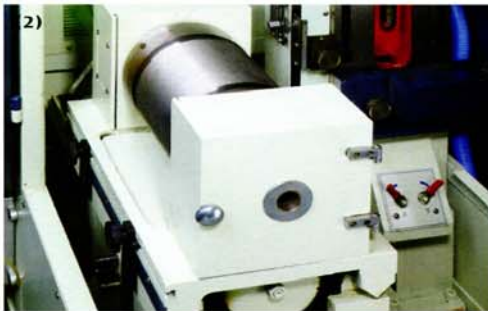
2) EFFICIENT FAST WIRE CUTTING THE WIRE BOBBIN DRIVING SYSTEM
